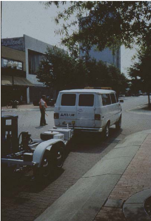
Figure VII: FWD testing utilized a Dynatest Model 8002 similar to the one pictured above
